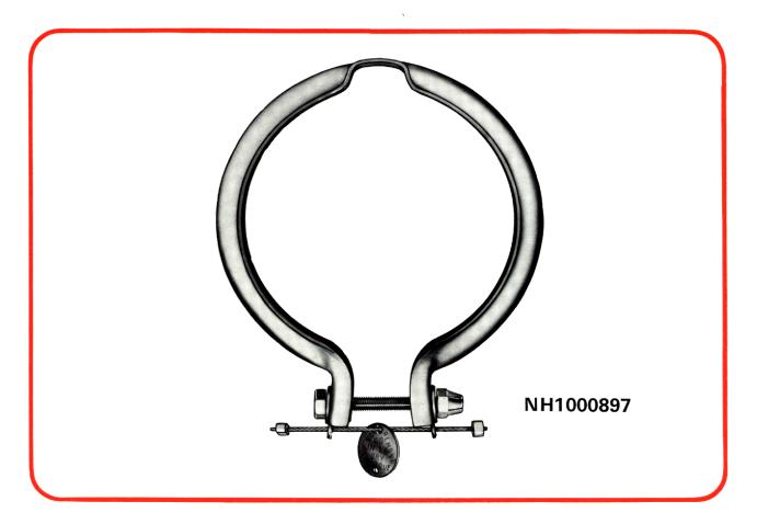
The Aeroquip NH1000897 clamp is now being used on a number of Cessna and Piper Aircraft as an exhaust connection. The high apex and spring design lugs accommodate thermal expansion caused by high temperature differential between hot internal exhaust gas and cooler ambient temperatures. The one-piece design eliminates welds or rivets which could cause failure
